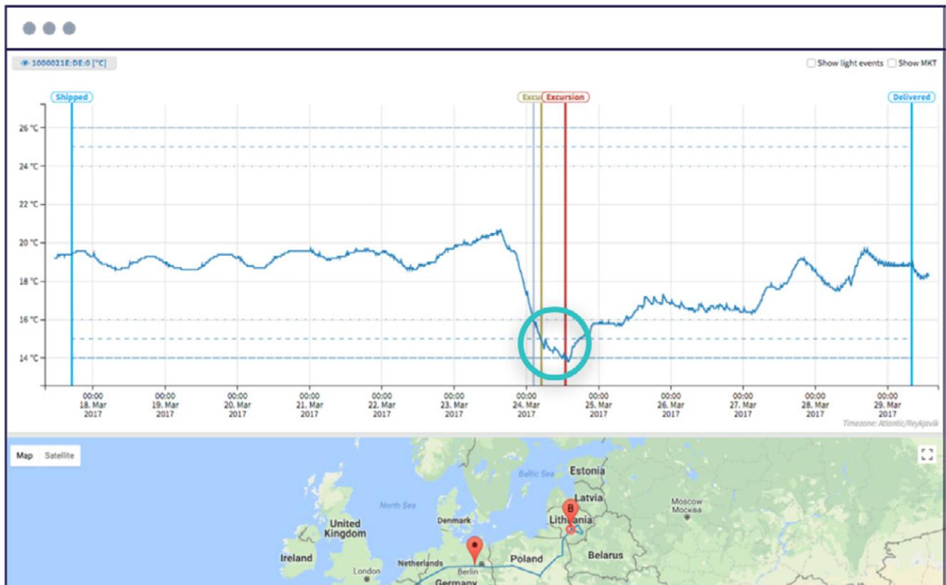
The truck maintained its own temperature monitoring system, which did not show that an excursion was occurring inside the truck. Upon closer inspection, it was discovered that a ventilation window located at the back of the truck had been left open, likely following a customs check.
